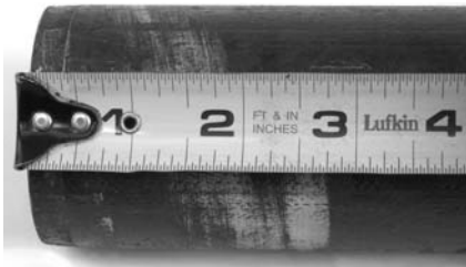
Figure 14C – Prep Area Not Square with End of Pipe
