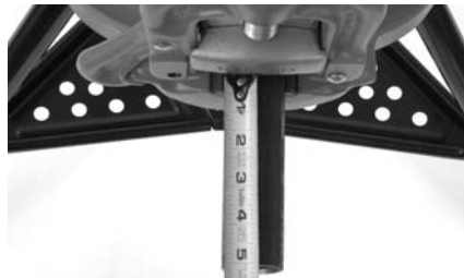
Figure 6 – Pipe In Vise, Inspecting For Adequate Prep Tool Clearance
