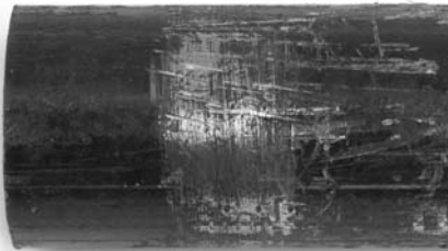
Figure 14A – Pipe Wrench Jaw Marks in Prep Area
